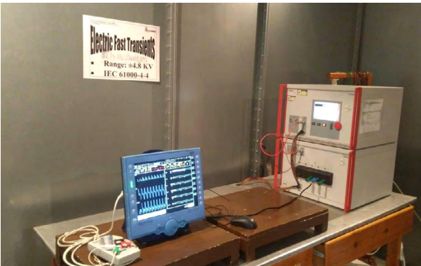
Fig. 31: Electrical Fast Transient (EFT) Test Setup
