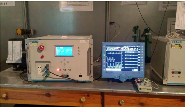
Fig. 32: Surge Immunity Test Setup
