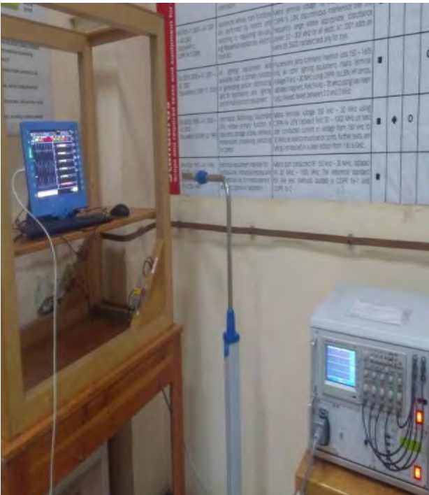
Fig. 34: Power Frequency Magnetic Field Setup
