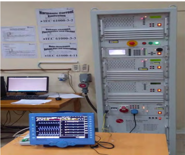
Fig.35: Voltage dips and short interruptions Setup
