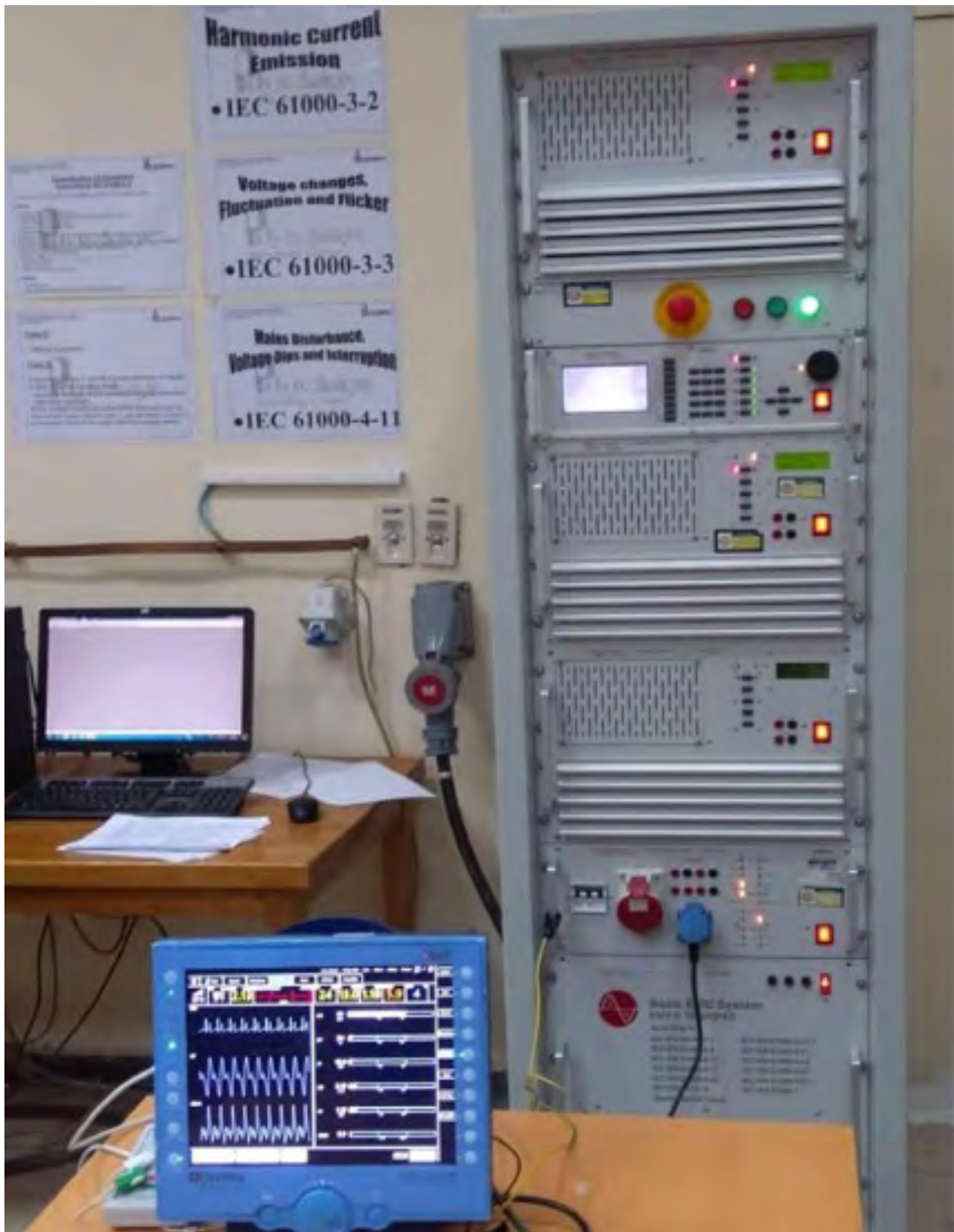
Fig. 27: Harmonic Current Emission Test Setup
